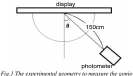
Fig.1 The experimental geometry to measure the gonio photometric characteristics
