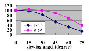
Fig.2 The gonio photometric characteristics of the LCD and PDP. In the figure, the values of the vertical axis are normalized as the luminance at 0 degree is 100. The luminance of the PDP at 0 degree is 236cd/m<sup>2</sup> and that of the LCD is 519cd/m<sup>2</sup>.
