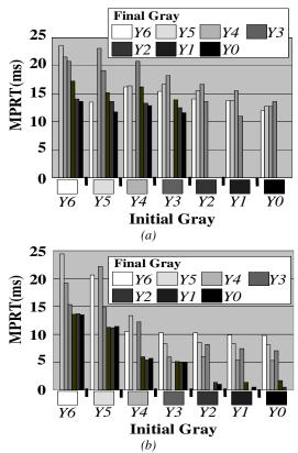
Fig. 3 The measured MPRT (a)LCD (b)PDP
