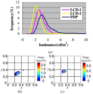
Fig.6 (a)~(c): The luminance histogram, xy chromaticity histogram (LCD-1) and xy chromaticity histogram (PDP) of Fig.5(a)
