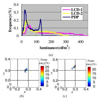
Fig.7 (a)~(c): The luminance histogram, xy chromaticity histogram (LCD-1) and xy chromaticity histogram (PDP) of Fig. 5(b).
